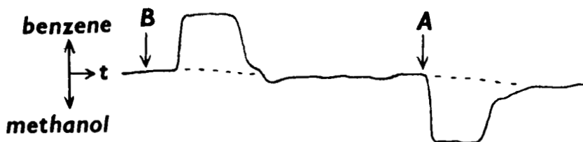
FIGURE 4 Example of the base line perturbations. Column: Silica gel CH-70, 70-200 \mu\text{m} , 25x0.6 cm I.D. Eluent: Benzene/methanol, azeotropic mixture. Pressure change: 5.3 MPa. Elution rate: 1.0 ml/min. Detector sensitivity: 32x. Symbols as in Fig. 2.
